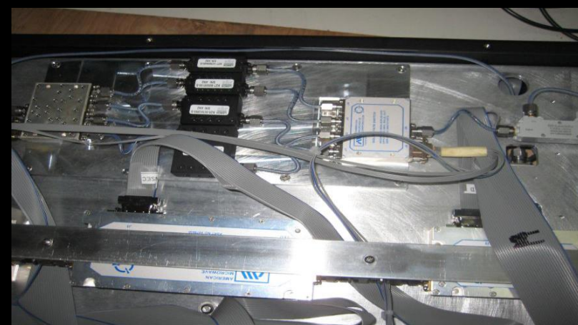
High Band Switched Filter Bank
