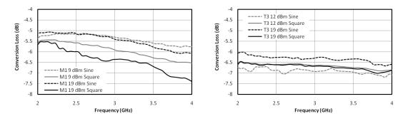
Fig. 6. Conversion loss for sine and square-wave LO for the M1 (left) and T3 (right) mixers. Notice that the M1 mixer is more sensitive to the LO, especially for high level drives. The T3 has a flatter, more robust conversion loss as a function of LO.
