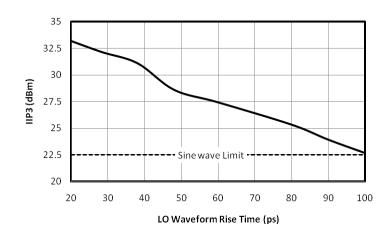
Fig. 12. IIP3 versus square-wave rise time.
