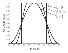
Fig. 2. The raised cosine pulse family. When  $\beta = 1$ , the pulse is a cosine function. When  $\beta = 0$ , the pulse is an ideal square with instantaneous rise time and 50% duty cycle.
