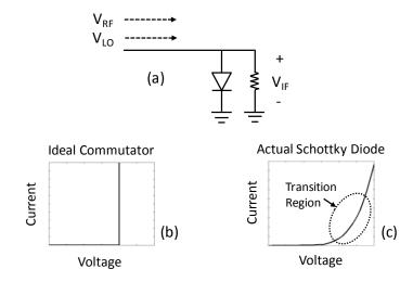
Fig. 1. (a) Simple single ended mixer. I-V characteristics for (b) the ideal commutator and (c) a realistic Schottky diode.
