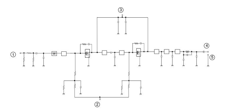
RoHS Compliance, 440-520MHz 7W 7.2V, 2 Stage Amp. For portable Radio
